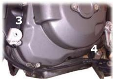
MOUNT THE THICKNESS H 10 IN CORRESPON-DENCE TO THE BRACKET 1USING THE 5X30 SCREW, USE THE RUBBER WASHER BETWEEN THE THICKNESS AND THE ENGINE SPOILER.
